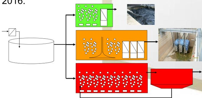
Figure 2a. RETROFIT Hybrid MBR plant (40 – 140 m<sup>3</sup>/day)
