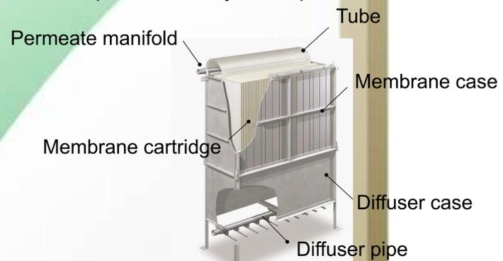
Figure 1. Kubota Submerged Membrane Unit structure
