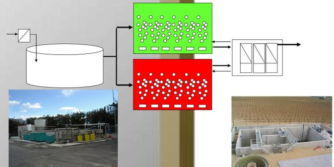
Figure 2b. NEW BUILD Modular MBR plant (70 - 224 m<sup>3</sup>/day)
